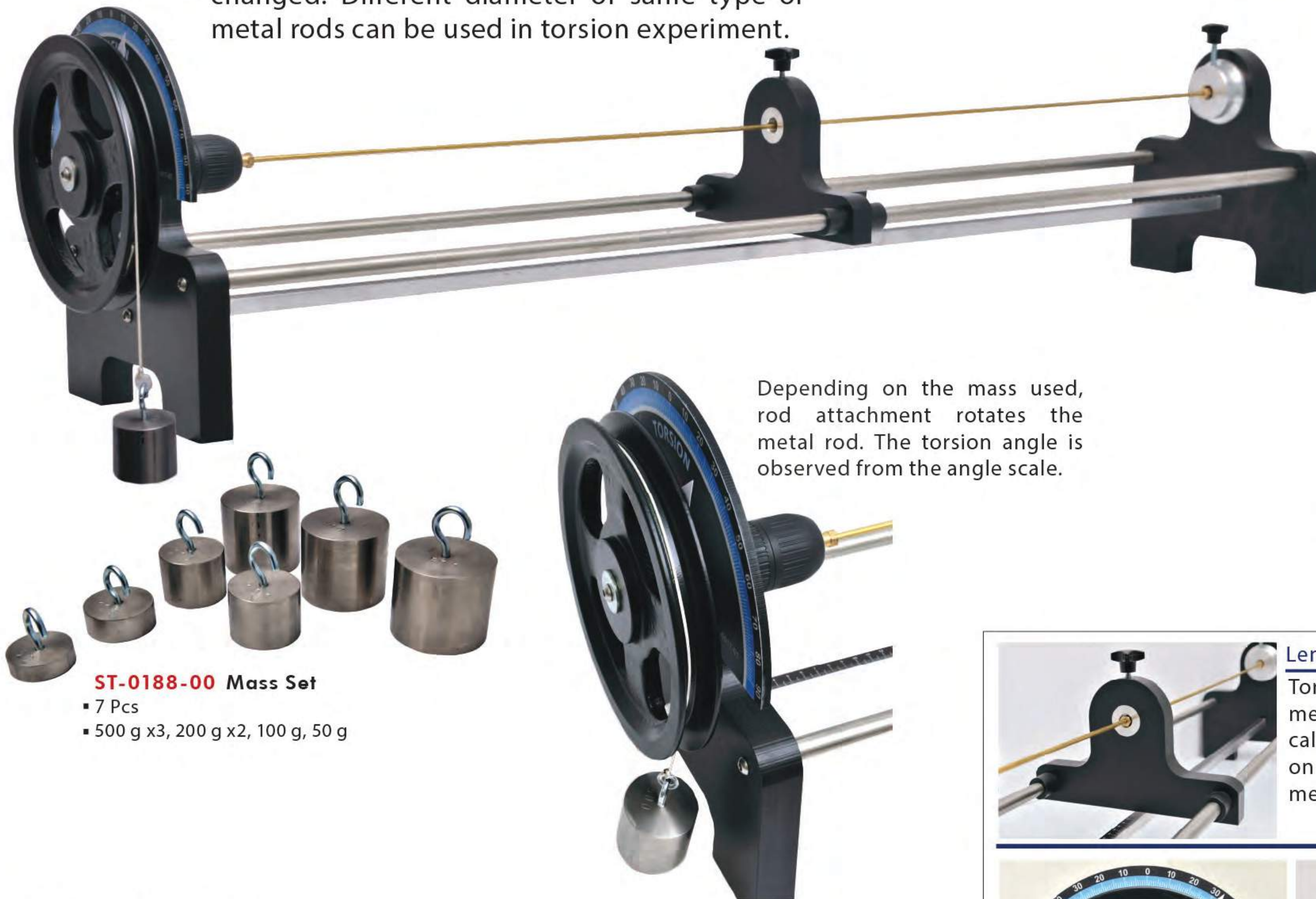
ST-0189-00 Metal Rods ■ 4 Pcs ■ Material Type: Brass and Stainless Steel ■ Diameter: 3 mm, 4 mm
