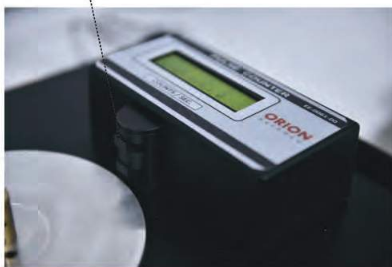
EE-0061-00 Pulse Counter Pulse counter (digital display) counts the numbers of bars of each disk at the same time
