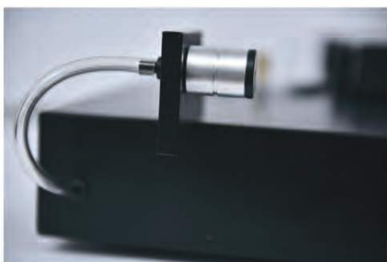
ME-0007-00 Frictionless Wheel The force in the string over the frictionless wheel causes a torque on the disks and they start to rotate
