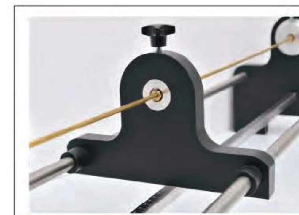
Length Adjustment Mechanism Torsion angle of half length of metal rods can also be calculated by fixing the screw on length adjustment mechanism.
