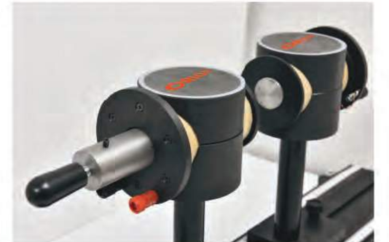
EE-0161-00 Solenoids The magnetic field on the germanium semiconductor is changed by the current supplied to the solenoids.
