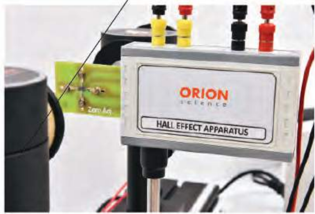
EE-0160-00 Hall Effect Apparatus Controlled voltage is applied to germanium crystal. Hall voltage is measured by multimeter.
