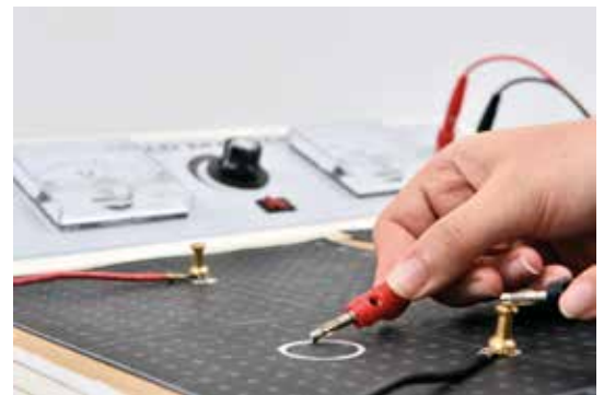
A conductive ring creates a region with equal potential on and inside the ring.
