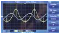
The screenshot of the oscilloscope shows a plot of the voltage applied on the solenoid and the voltage induced in the small coil.
